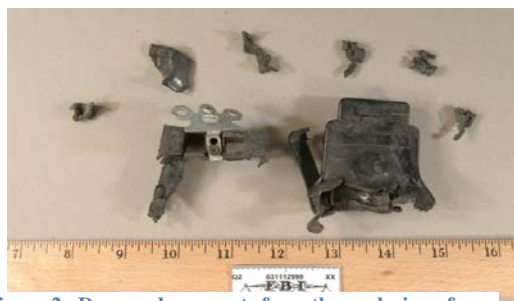
Figure 2. Damaged remnants from the explosion of an IED that are visually consistent with the body of an electrical timer.
