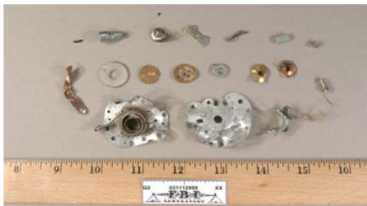
Figure 1. Damaged remnants from the explosion of an IED that are visually consistent with the internal components of an electrical timer.
