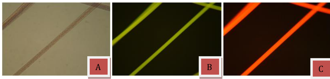
Figure 2: Images of the same set of fibers viewed with A) transmitted light microscopy; B) fluorescence microscopy using 450nm-490nm excitation; C) fluorescence microscopy using 510nm – 560nm excitation.
