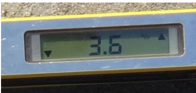
Measurement of cross slope.
