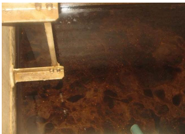
Soot collection tank that held oily waste prior to overboard discharge
