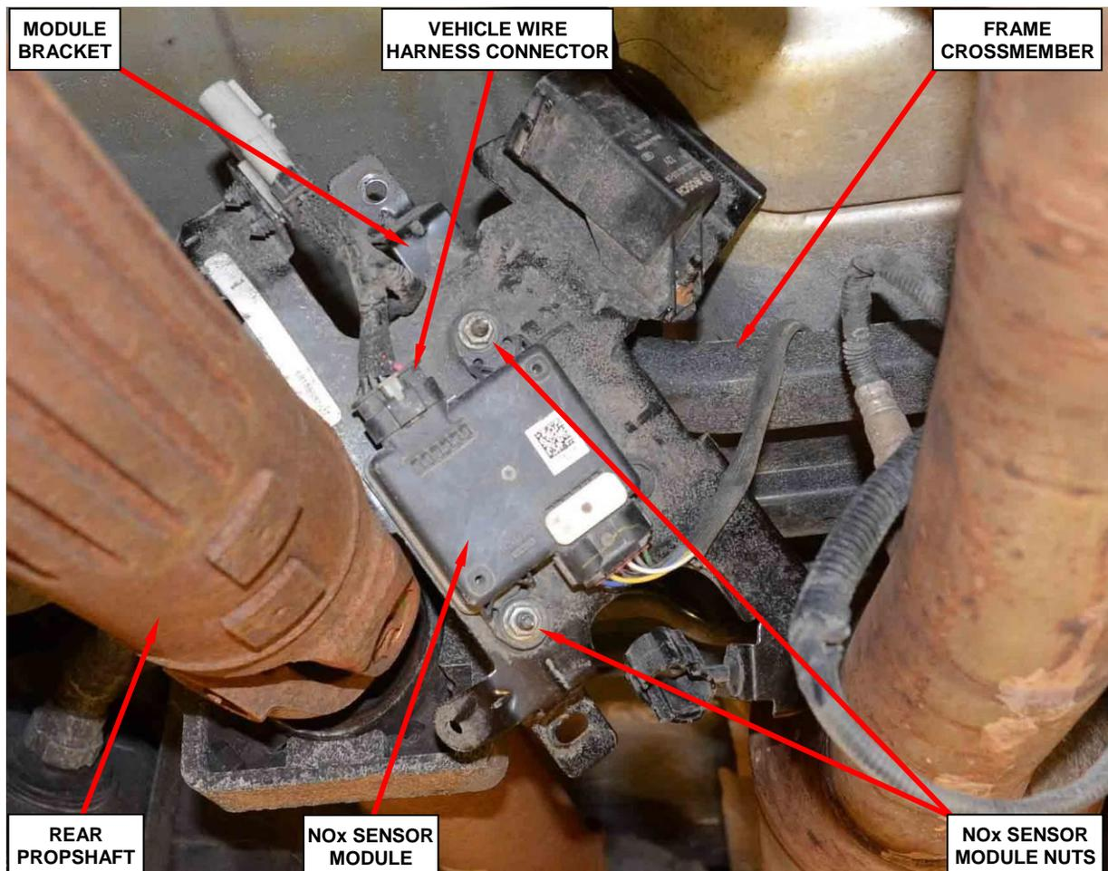
**Figure 26 – NO<sub>x</sub> Sensor Module**
