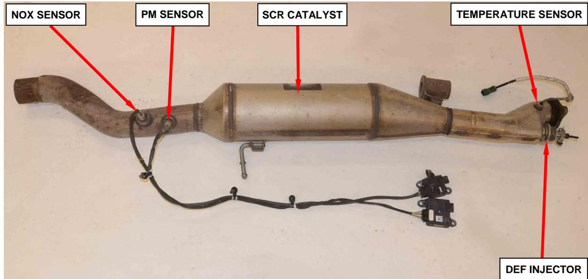
**Figure 15 – Selective Catalytic Reduction (SCR) Catalyst Assembly**
