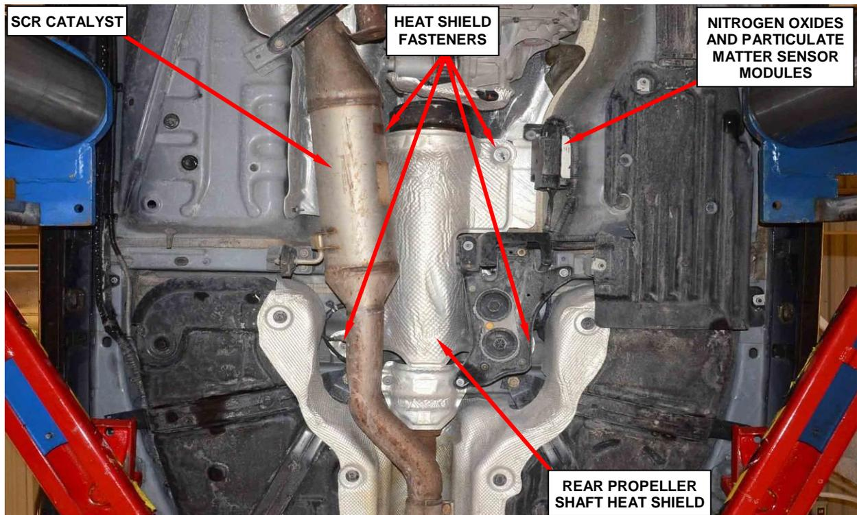
**Figure 7 – Rear Propeller Shaft Heat Shield**
