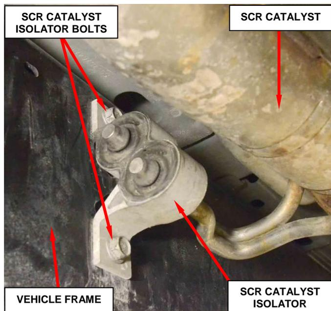
Figure 29 – SCR Catalyst Isolator
