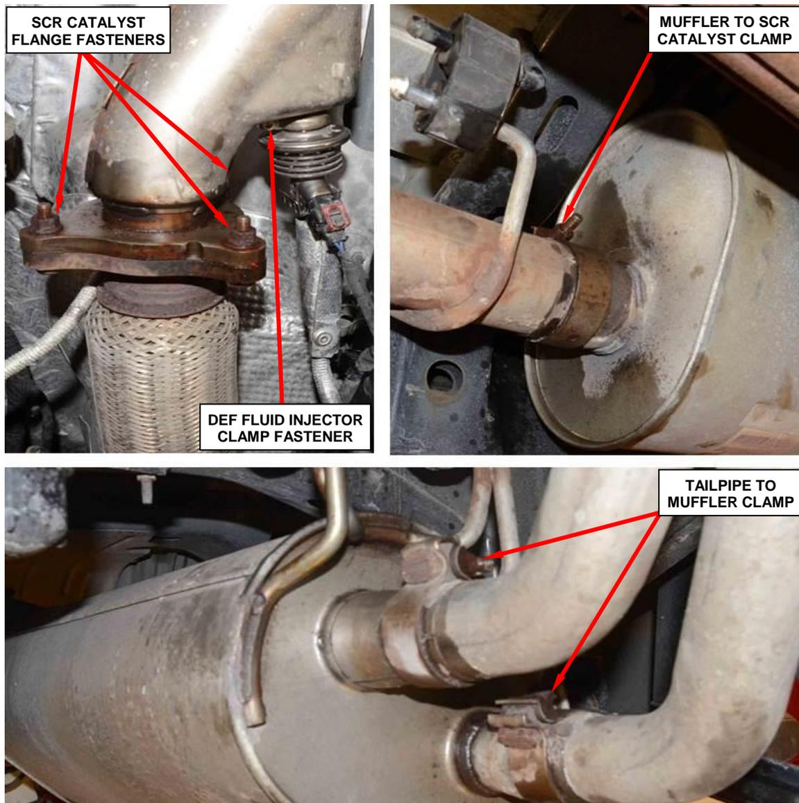
**Figure 19 – Saturate Exhaust Fasteners with Penetrating Lubricant**
