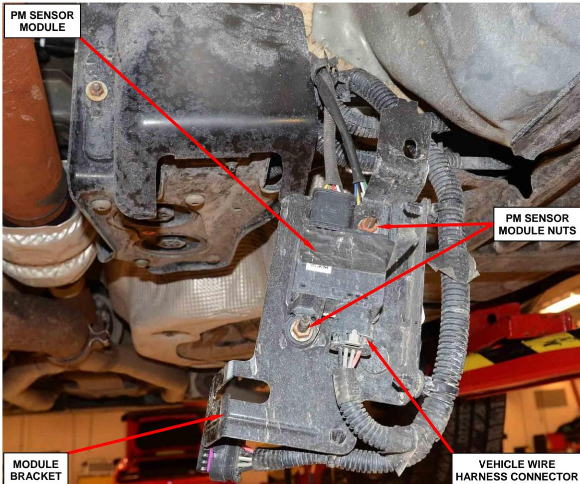
**Figure 10 – PM Sensor Module**
