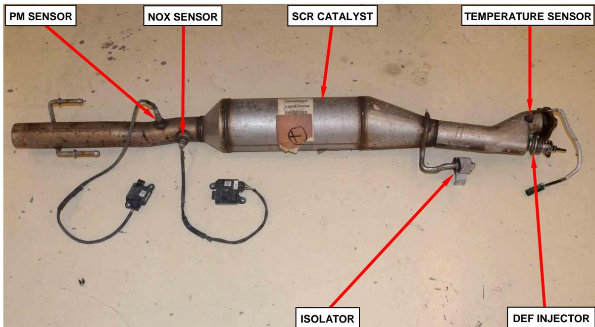
**Figure 32 – Selective Catalytic Reduction (SCR) Catalyst Assembly**
