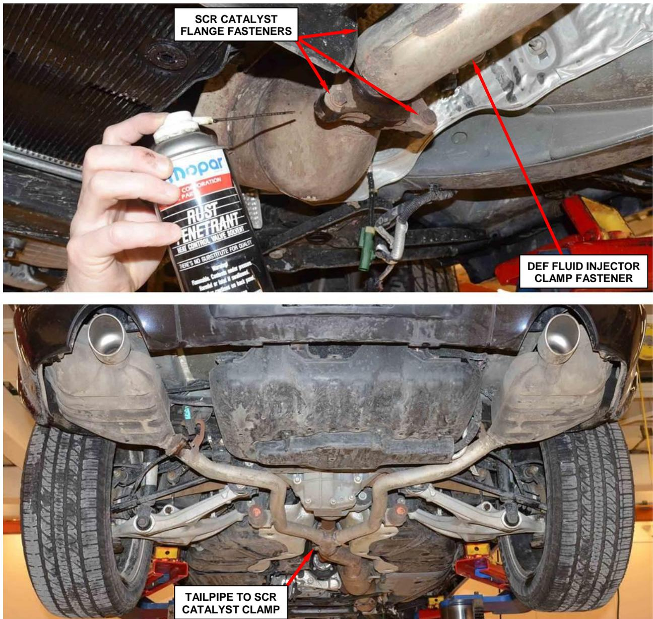
**Figure 3 – Saturate Exhaust Fasteners with Penetrating Lubricant**
