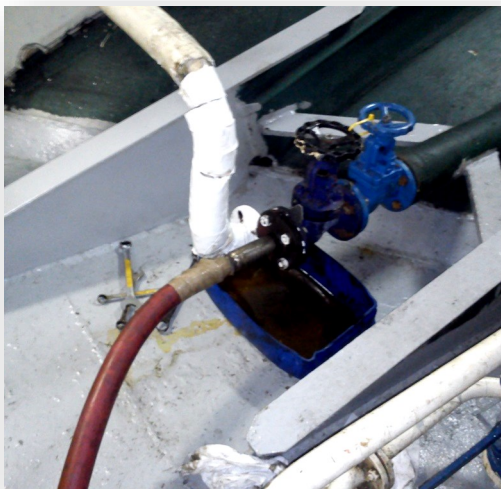
"Magic Hose" connected to overboard discharge valve
