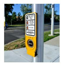
An Accessible Pedestrian Signal (APS), pictured here, is a device attached to a pole at a signalized intersection that communicates information about when and where it is safe to cross a street in an audible and vibrotactile manner so that individuals who are blind or deafblind have access to the same crossing information as sighted pedestrians. *Id.* ¶17. An APS has a round
