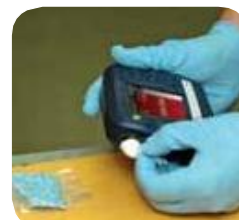
Analyze through sealed packaging for most samples.
