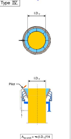
Where: A<sub>tip-unob</sub> = Unobstructed Cross Sectional Area of Flare Tip
