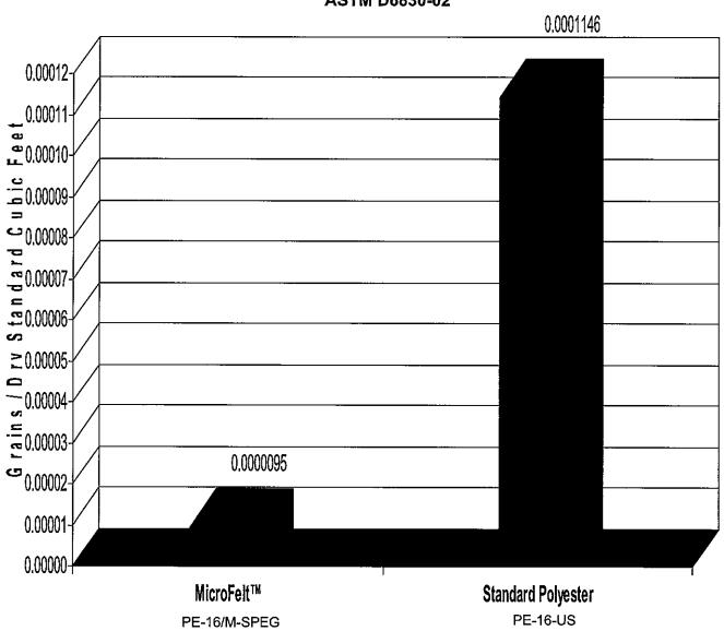
NOTE: TEST DUST PARTICLE SIZE DISTRIBUTION: 77% LESS THAN 2.5 MICRON
