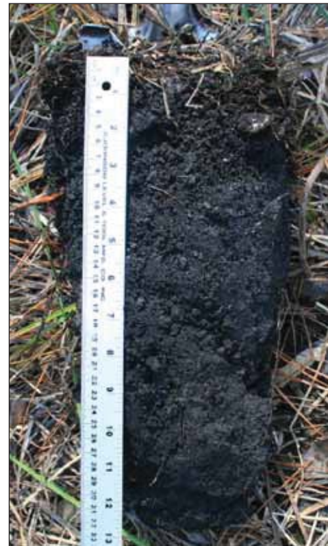
Figure 19. Example of indicator S7 (Dark Surface) in a sandy soil. Scale in inches on right.
