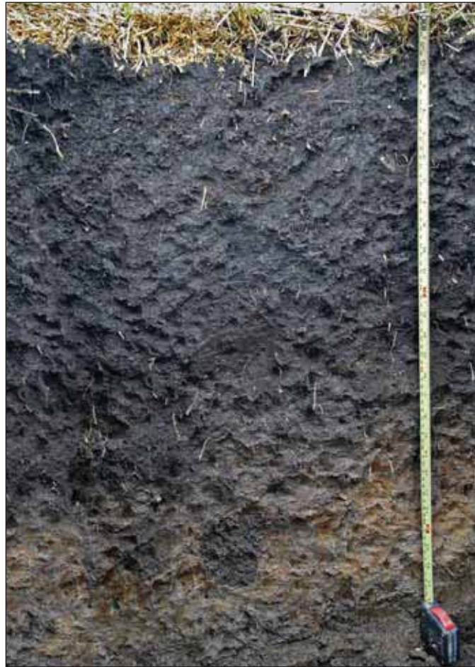
Figure 13. Deep observations may be necessary to identify the depleted or gleyed matrix below a thick, dark surface layer. In this example, the depleted matrix starts at 20 in. (50 cm).
