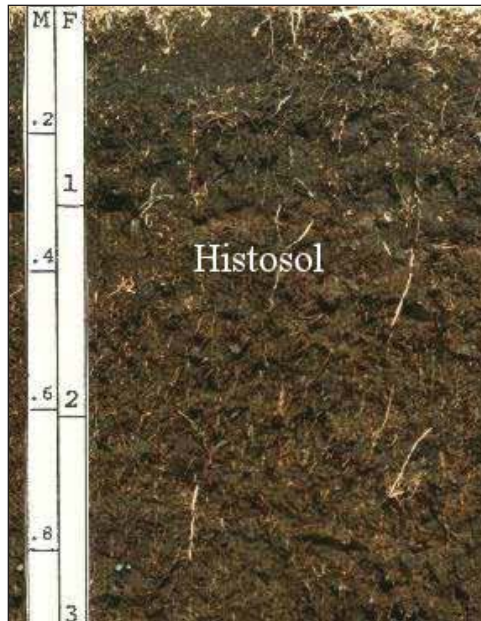
Figure 7. Example of a Histosol, in which muck (sapric soil material) is greater than 3 ft (0.9 m) thick.
