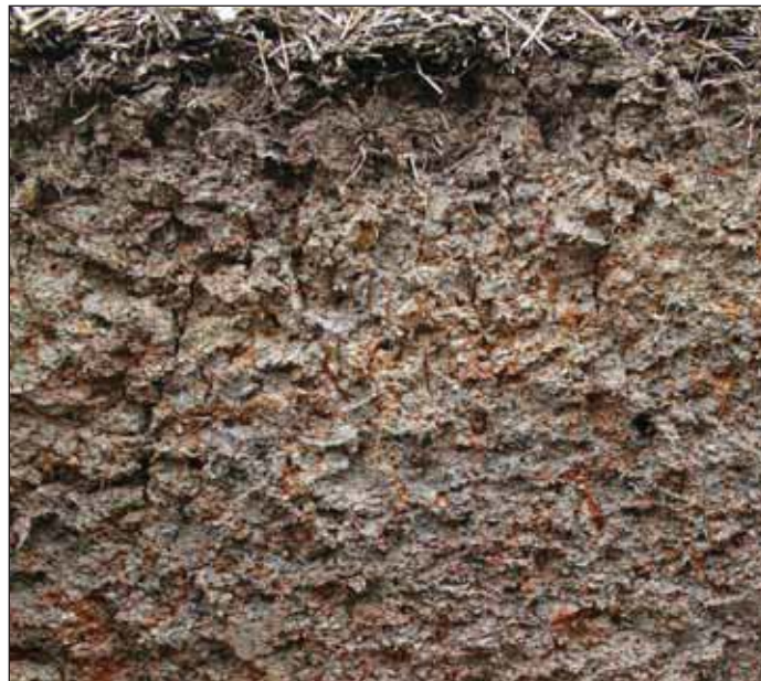
Figure 23. Example of indicator F3 (Depleted Matrix), in which redox concentrations extend nearly to the surface.
