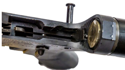
Image depicting a “Lightning Link,” which is designed to be installed in the fire-control cavity of an AR-15 type receiver.
