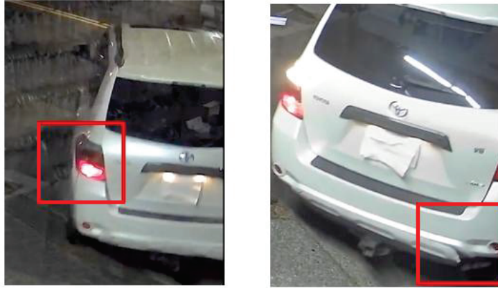
White Toyota Highlander with vertical crack on driver's side rear bumper caused by impact with the pharmacy (left) and pre-existing damage on the passenger side (right)
