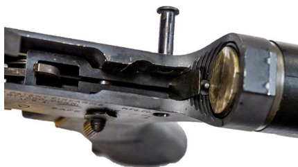
Image depicting a “Lightning Link,” which is designed to be installed in the fire-control cavity of an AR-15 type receiver.
