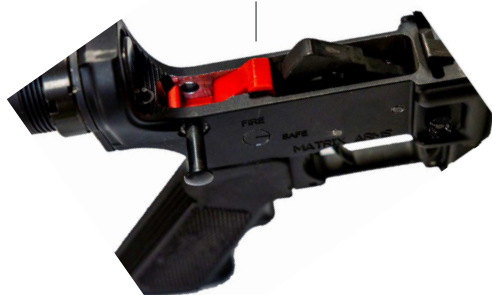
Images depicting 3D printed “Swift Links,” which are designed to be installed in the fire-control cavity of an AR-15 type receiver.
