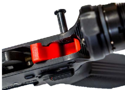
Images depicting 3D printed “Swift Links,” which are designed to be installed in the fire-control cavity of an AR-15 type receiver.
