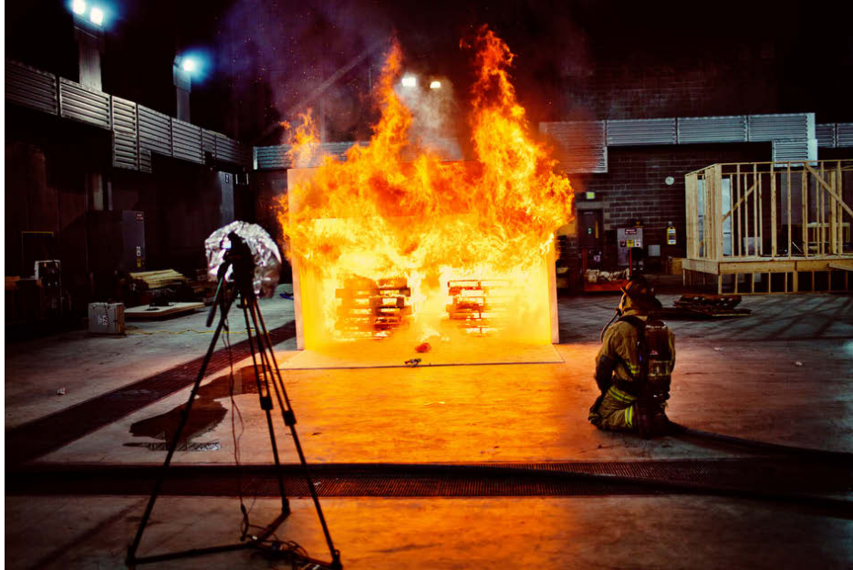
A demonstration cell burns to test a newer, thinner drywall at the ATF Fire Research Laboratory.
